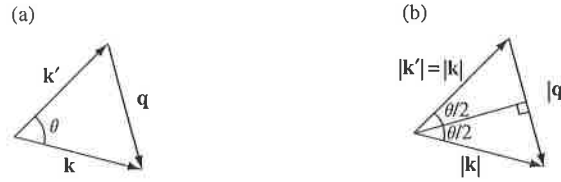
Fig. 8.10 (a) Diagram illustrating initial wave vector \mathbf{k} , final wave vector \mathbf{k}' , and transferred momentum \mathbf{q} . To indicate that momentum is transferred from the incident particle we choose the convention \mathbf{k} = \mathbf{k}' + \mathbf{q} . (b) For elastic scattering, the scattered angle \theta is related to q by k \sin(\theta/2) = q/2 .
